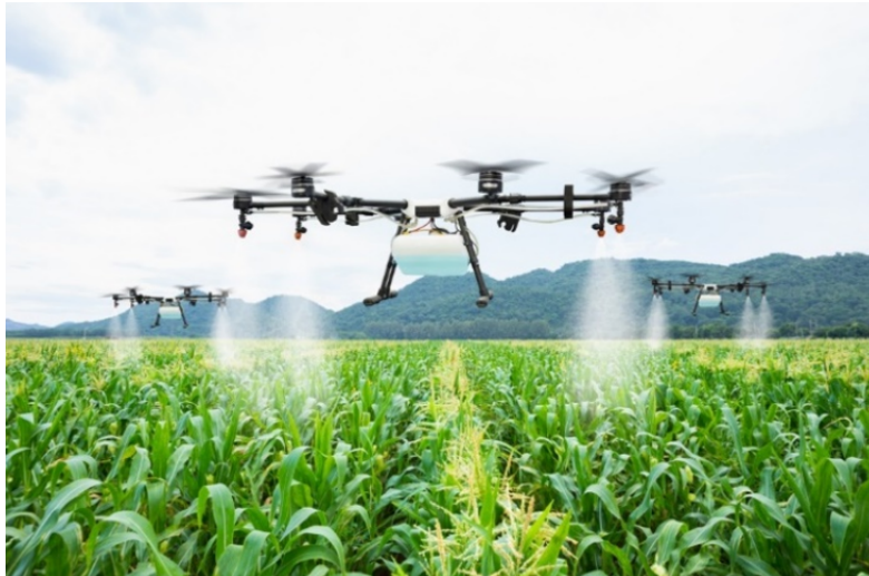
Fig. 2. Process of a drone spraying
