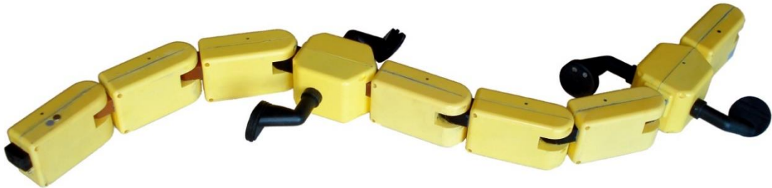
Figure 1. The robot developed by Auke Jan Ijspeert and colleagues, which walks and swims like a salamander. Credits: Kostas Karakasiliotis, Biorobotics Laboratory, EPFL, Lausanne.
