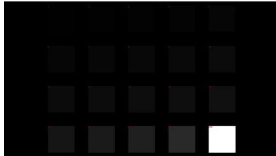
Fig. 5. Test image for additional black level adjustment of the projector
