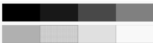
Fig. 1. Test image for calibration of projector before measurements according to GOST IEC 61947-1-2014 [13]
