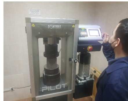
b) Compressive strength test
