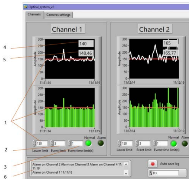
Figure 8. Program interface: 1 – threshold value, 2 – number of triggers, 3 – trigger time period, 4 – average amplitude value, 5 – instantaneous amplitude value, 6 – response time fixation window.
