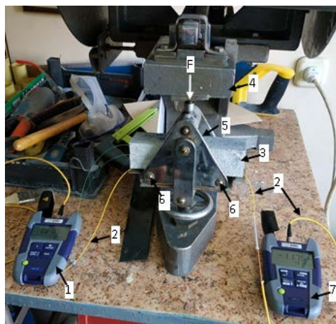
Figure 5. Testing machine MII – 100 (two-support bend): 1 – radiation source; 2 – optical single-mode fiber in a protective sheath; 3 – beam; 4 – testing machine MII-100; 5 – area of pressure application; 6 – stationary support; 7 – optical power meter.
