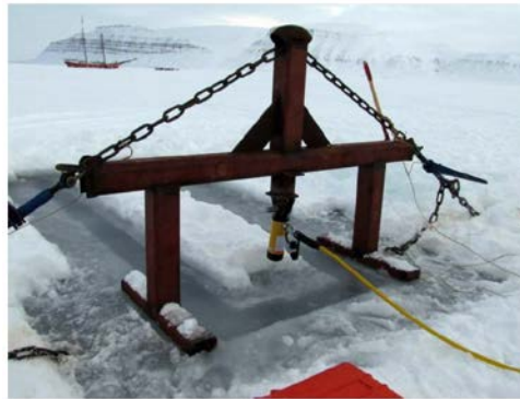
Figure 2. Field experiment to determine the bending strength of a beam [12].
