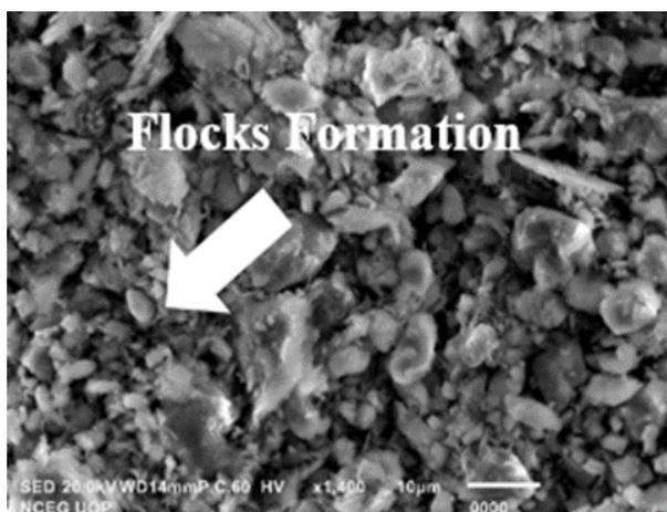
Figure 10 Untreated Sample (10 micrometer).
