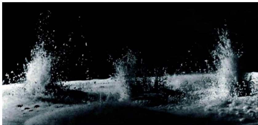
Figure 10. Loud sound (large amplitude), lifting the powder up (Jenny, 2001, p. 69)
