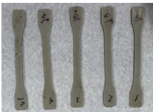
Fig. 1. Dumbbell-shaped specimens for testing
