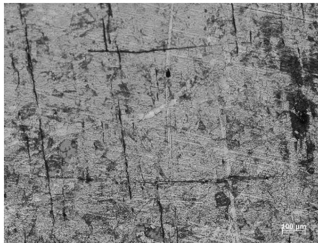
Fig. 6. Spall and shear cracks in steel ( \times 100 )
