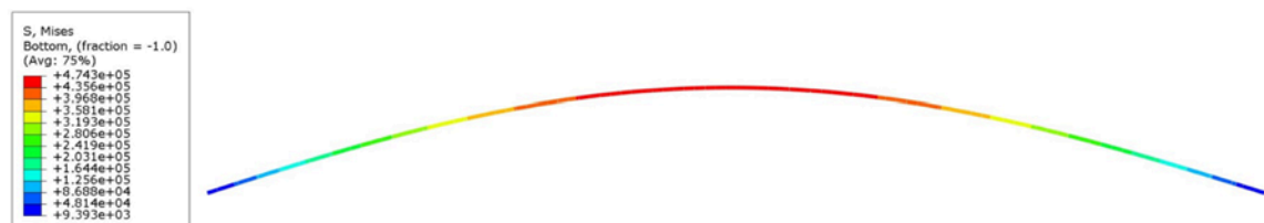
Fig. 3. Equivalent stresses calculated in Abaqus
