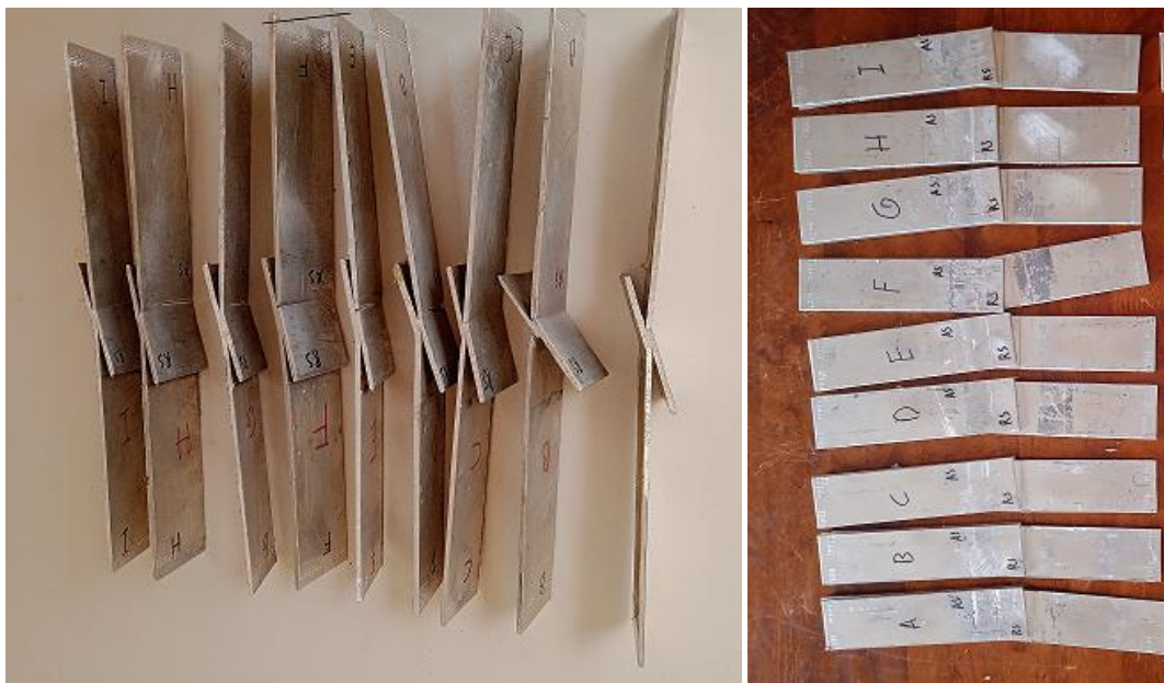
Fig.10. Different modes of fracture: a) single lap; b) double lap
