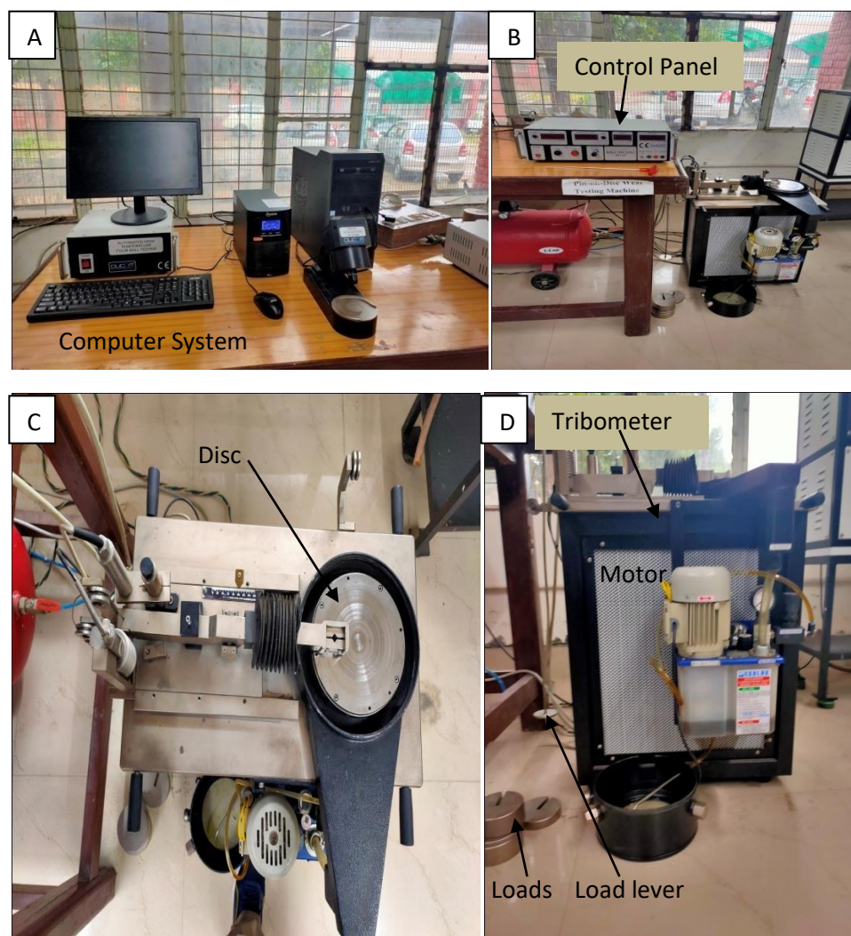
Fig. 6. Tribometer pin on disc: DUCOM make (A) System attached to pin on disc tribometer. (B) Control Panel of pin on disc. (C) Top view of pin on disc tribometer. (D) Front view of pin on disc tribometer.
