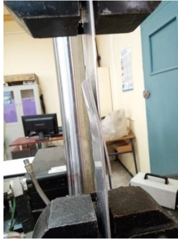
Fig.9. Shear specimen during the tensile test
