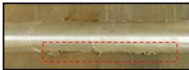
Fig. 4. Burrs after welding FSW.
