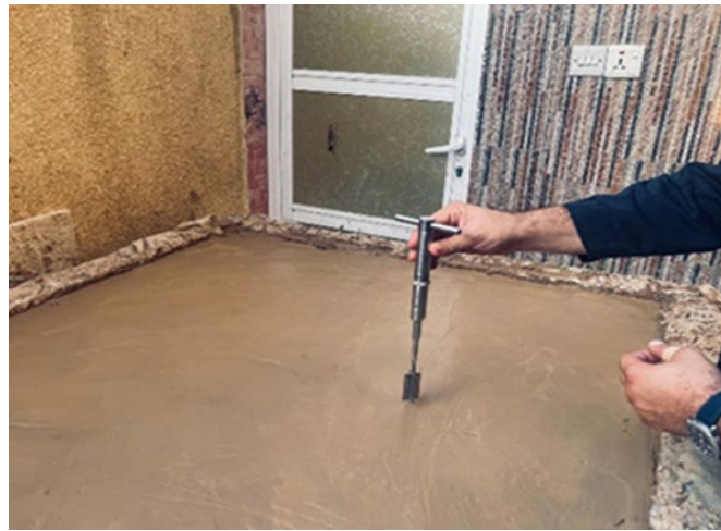
Figure 4. A portable vane shear device is used to control the undrained shear strength.
