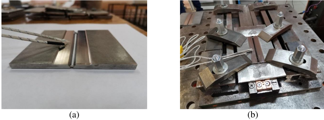
Fig. 2. Places for installation of "K-type" thermocouples on a welded sample 100 \times 100 \times 4 mm (a) and equipment for welding sheet blanks (b)
