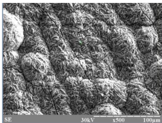
Fig. 3. Structure of the modified coating at a concentration of \text{Cr}_2\text{O}_3 in the electrolyte of 20 g/l
