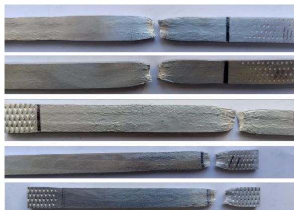
Fig. 10. Fractures tensile tests samples of the 226-233 (top to bottom) samples
