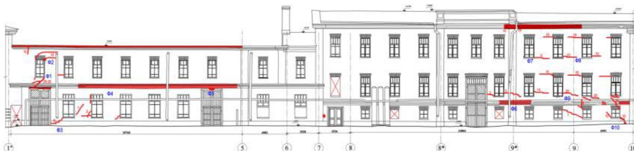
Figure 22. Scheme of building facade defects 6 .
