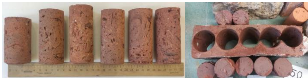
Figure 10. Cylindrical samples prepared for TXT and UCT, compiled by the authors.
