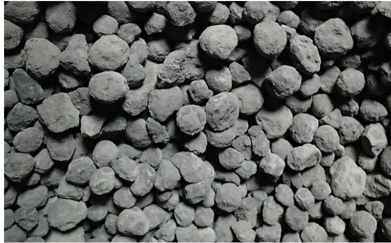
Figure 2. Portland cement clinker appearance.
