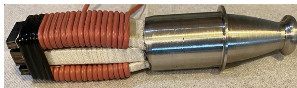
Figure 3. Experimental sample of a magnetostrictive transducer.
