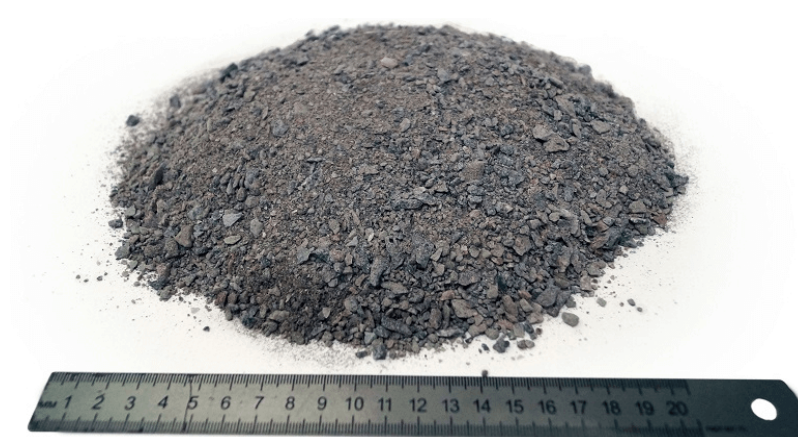
Figure 6. Screenings of crushed granite.
