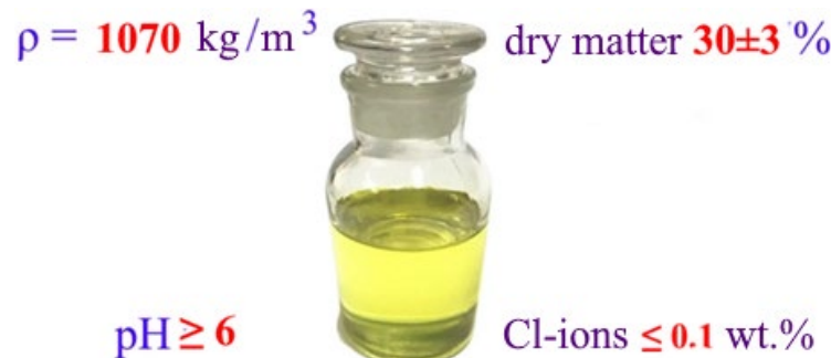
Figure 7. The superplasticizer characterization.
