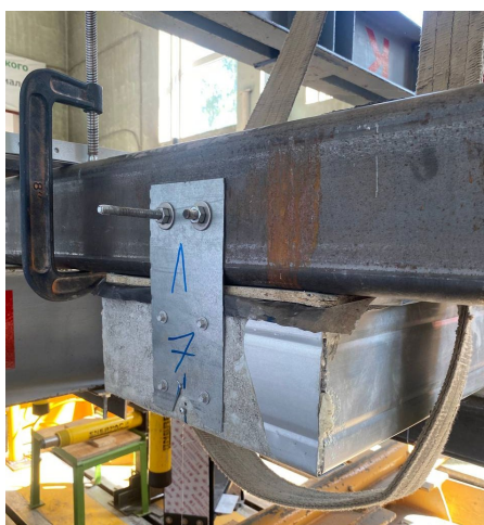
Figure 7. Fastening of the panel before the start of the test.
