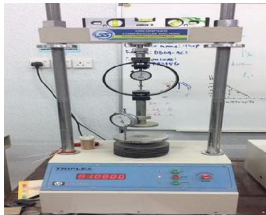
Figure 3. The specimen was compressed under UCT machine.
