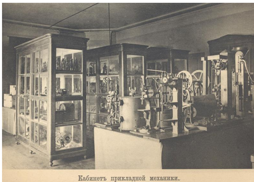
Figure 1. Collection of kinematic models for teaching the course Applied Mechanics at IMTS, Moscow, postcard circa early 20th century.
