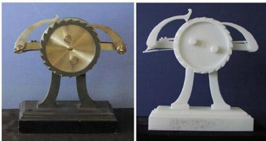
Figure 4. A ratchet mechanism with three spring-loaded stoppers (a) Original Reuleaux model, (b) Rapid prototype model (Lipson et al., 2005).
