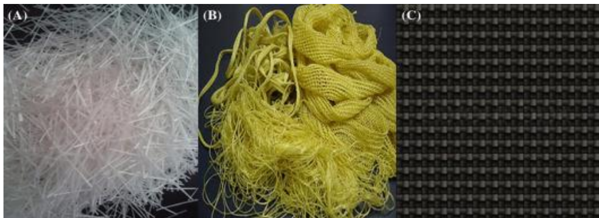
Fig. 7. Displaying synthetic fibers (A) glass, (B) kevlar, and (C) carbon fibers. Reprinted with permission from [24], © Elsevier 2017
