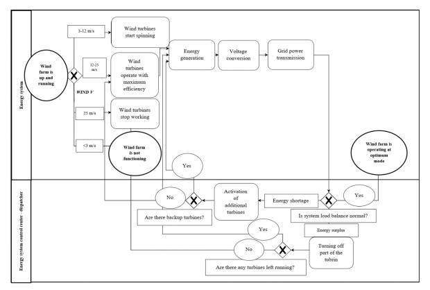
Fig. 3. Wind farm process before digitalization in BPMN notation (designed by the author).
