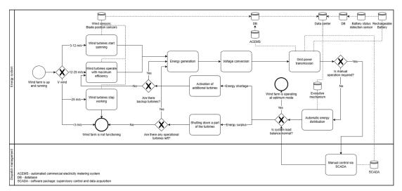
Fig. 4. Wind farm operation process after digitalization in BPMN notation (designed by the author).
