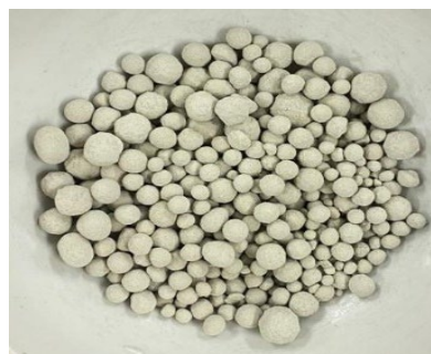
Figure 4. Granulated aggregate, obtained in a laboratory facility.
