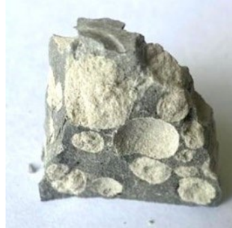
Figure 8. Mortar sample chipping with granular aggregate 10 mm fractions.
