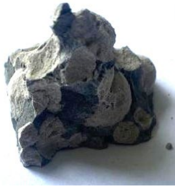
Figure 7. Mortar sample chipping with granular aggregate 5 mm fractions.
