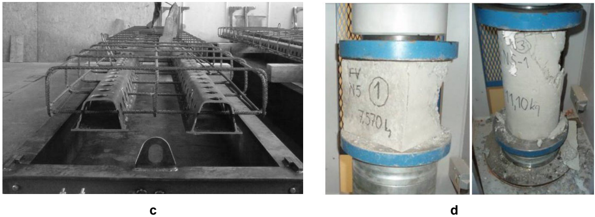
Figure 9. Experimental testing of the pedestrian bridge slab: general view of the testing bench (a), load application scheme (b), reinforcement frame (c), testing the cube and cylinder strength of concrete specimens (d).
