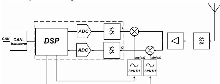
Fig. 2. The structural scheme of the AIS receiver.
