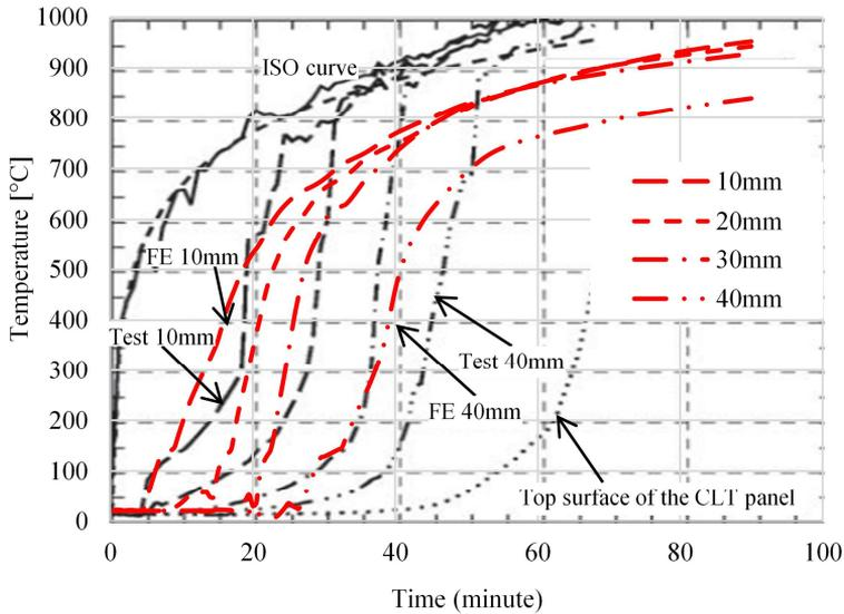
**Fig. 5.** Comparison between measured temperatures for the fire tests V2 [8] and numerical simulation with the assumption that charred layers immediately fall off after charring.
