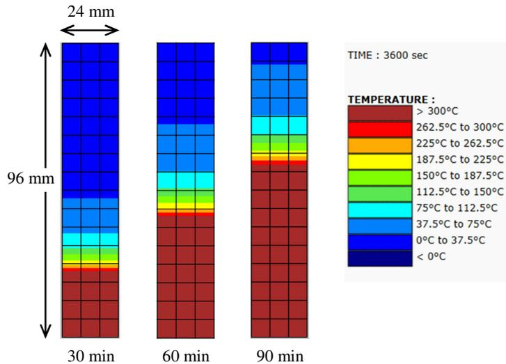
Fig. 1. Temperature distributions within the cross-section of solid timber after 60 minutes of fire exposure.
