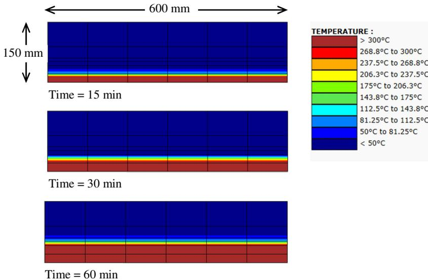
**Fig. 3.** Numerical temperature profiles across the cross section of CLT and the formation of charring layer at different fire-exposure times.
