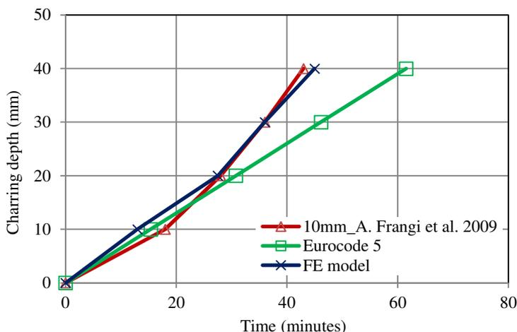
**Fig.7.** Charring depth for CLT panel measured from test [8] and compared with EN 1995-1-2 [6] and numerical model.
