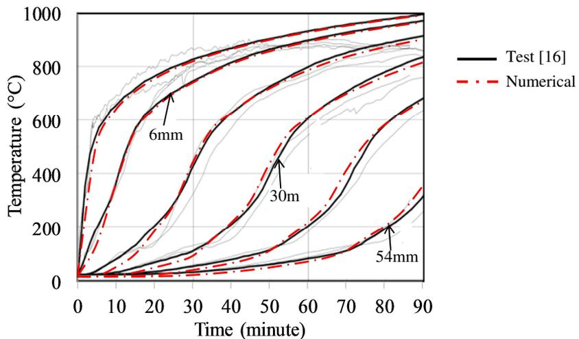
Fig. 2. Experimental [16] and numerical temperature distributions at various depth across the cross section of solid timber.
