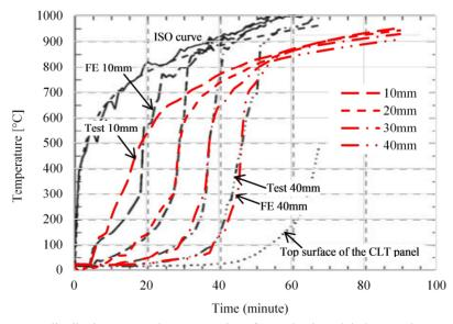
Fig.6. Temperature distributions across the cross-section of cross-laminated timber panels - experimental and numerical.
