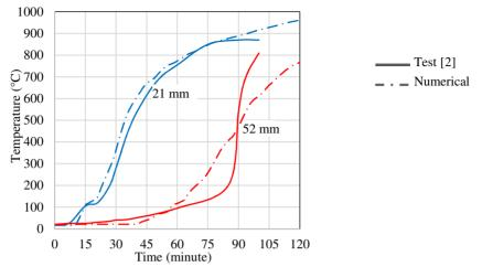
Fig. 4. Comparison between predicted and measured temperatures for CLT panel in fire.
