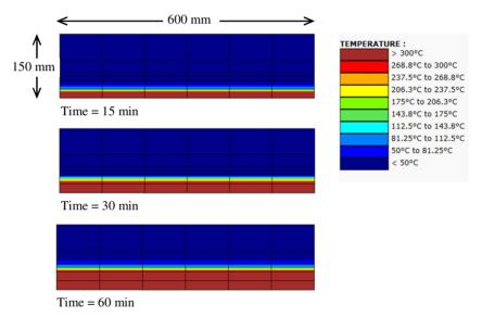
Fig. 3. Numerical temperature profiles across the cross section of CLT and the formation of charring layer at different fire-exposure times.
