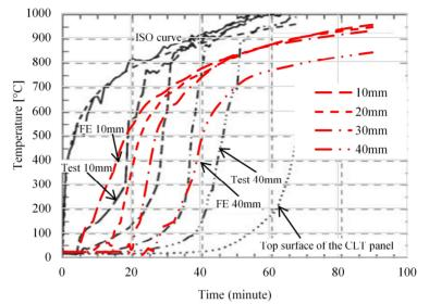
Fig. 5. Comparison between measured temperatures for the fire tests V2 [8] and numerical simulation with the assumption that charred layers immediately fall off after charring.
