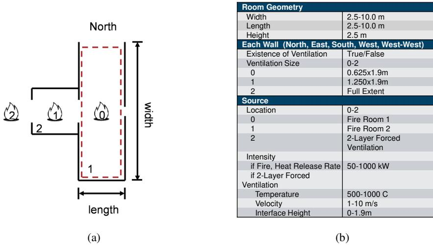
Fig. 4. The two-room configuration used to generate data sets with FDS.
