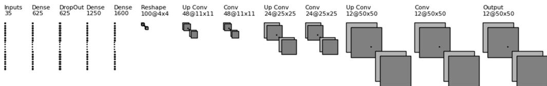
Fig. 5. Up-convolutional neural network used to predict fire spatial fire conditions from network model input data.
