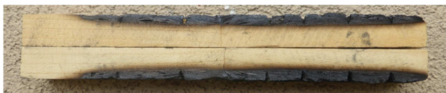
Fig. 7. Charred layer – vertical finger joints.
