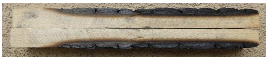
Fig. 8. Charred layer – horizontal finger joints.
