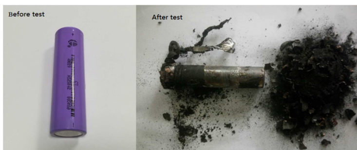
Fig. 2. The picture of the sample cells before and after the EV-ARC test. After the test the cell can ruptured and some broken electrodes ejected from the cell.
