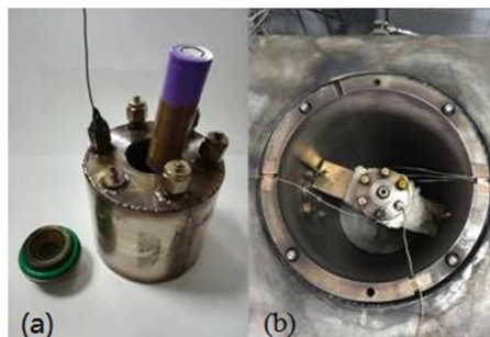
Fig. 1. The illustration of the canister (a) [15] and the final test apparatus in the EV-ARC (b).
