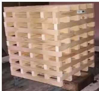
Fig. 2. Fire source in the experiments (overlapping wooden slats).
