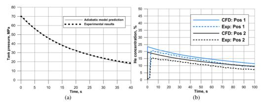
**Fig. 5.** Experimental and numerical predictions. (a) Storage pressure dynamics; (b) Helium concentration at plate surface sensors
