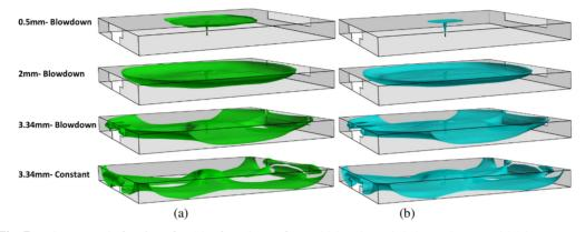
**Fig. 7** Hydrogen mole fraction after 20 s for releases from 700 bar through 0.5 mm, 2 mm and 3.34 mm TPRD diameters. (a) Iso-surface 1% vol; (b) Iso-surface 2% vol.
