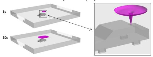
**Fig. 11.** Iso-surface showing 4% hydrogen mole fraction an *upward* release from 700 bar through a 0.5 mm TPRD.
