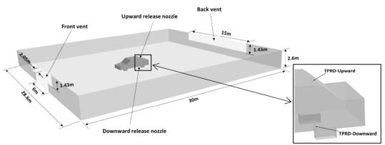
Fig. 1. Sketch of the naturally ventilated covered carpark with car geometry. Insert highlights TPRD location.
