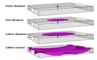
**Fig. 8.** Iso-surface showing 4% hydrogen mole fraction after 20 s for releases from 700 bar through 0.5 mm, 2 mm and 3.34 mm TPRD diameters.
