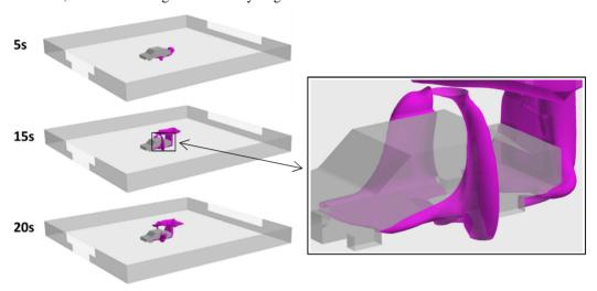
**Fig. 10.** Iso-surface showing 4% hydrogen mole fraction for a *downward* release from 700 bar through a 0.5 mm TPRD.
