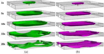
**Fig. 6.** Hydrogen mole fraction for a constant release of 0.299 kg/s through a 3.34 mm diameter TPRD. (a) Iso-surface 1% vol; (b) Iso-surface 4% vol.
