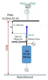
Fig. 4. Schematic diagram of KIT experiment for an impinging helium jet.
