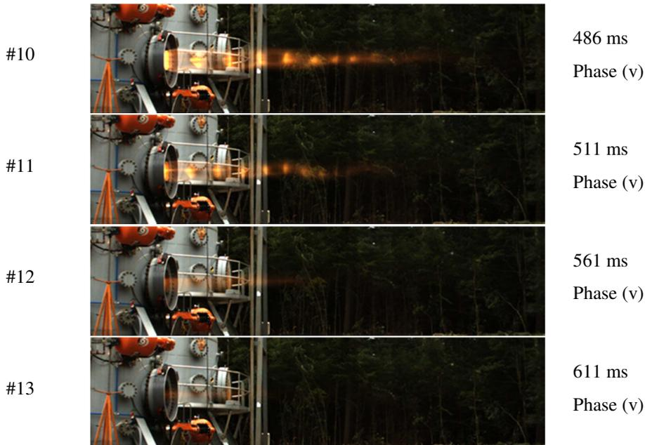
**Fig. 4.** Image sequence from a selected 400-mm orifice test (Vented-400-2) showing external flame.
