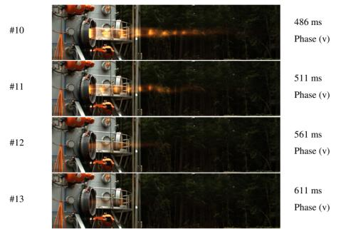
Fig. 4. Image sequence from a selected 400-mm orifice test (Vented-400-2) showing external flame.
