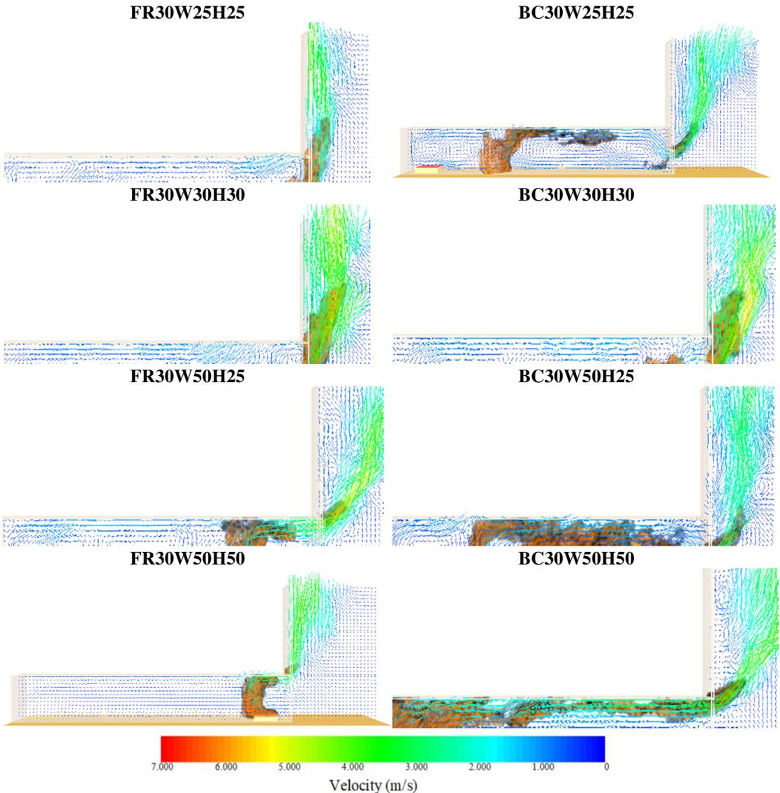
**Fig. 8.** Predictions of velocity vectors and flame envelope 900 s after fire initiation, corresponding to *Region III*, for all test cases.
