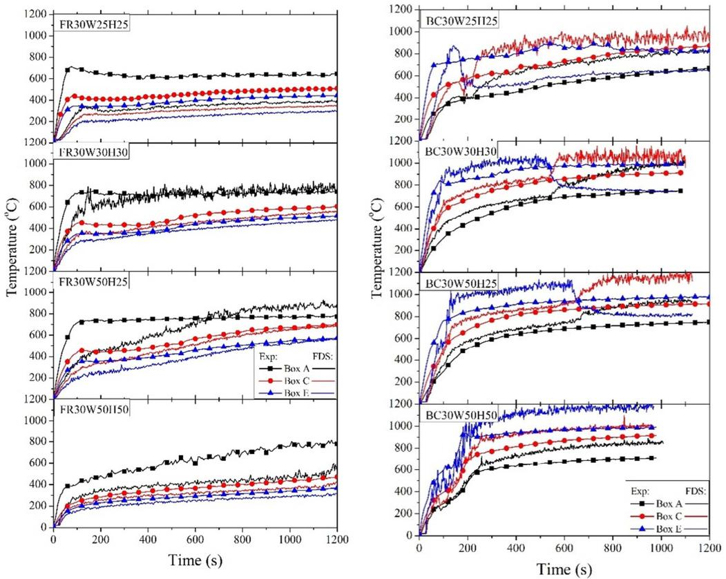
**Fig. 7.** Experimental and numerical temporal evolution of the gas temperature at a height of 45 cm in the interior of the corridor in Boxes A, E and E for FR (left) and BC (right) test cases.
