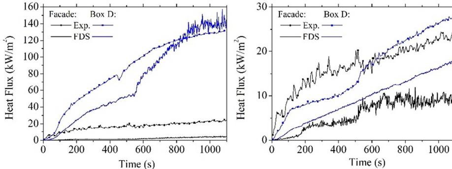
**Fig. 6.** Predictions and measurements of the temporal evolution heat fluxes for test cases BC30W30H30 (left) and FR30W30H30 (right).
