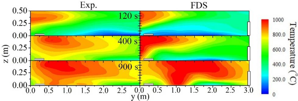
**Fig. 4.** Spatial distribution of the gaseous temperature at the corridor interior (BC30W30H30).
