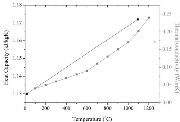
**Fig. 3.** Temperature-dependent values of heat capacity and thermal conductivity for the fibreboards used in the compartment's walls.
