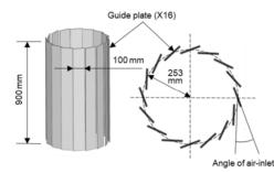
Fig. 1. Schematic for the fire tubular device.
