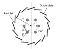
Fig. 2. Location of six fire sources on the bottom board of the tubular device. D is the diameter of fire source (mm), r is the distance from the tubular device center to a fire source (mm), R is the distance from the center of the tubular device to the center of a guide plate (mm), S is the distance between fire sources (mm).
