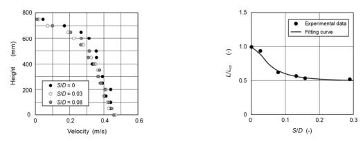
Fig. 9. Velocity of crosswind through the air inlet.
