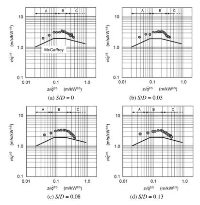
**Fig. 8.** Upward velocity of hot current along the central axis of fire source. A – continuous flame region; B – intermittent flame region; C – plume region.
