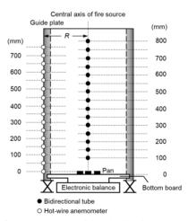
Fig. 3. Arrangements of the bi-directional tubes and hot-wire anemometers in the tubular device.
