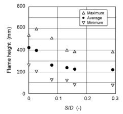
Fig. 6. Flame height change as a function of S/D.
