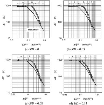
**Fig. 7.** Temperature attenuation along the central axis of fire source. A – continuous flame region; B – intermittent flame region; C – plume region.
