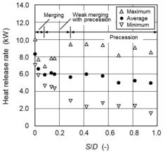
Fig. 4. Variation of heat release rate compared to ratio of distance between fire source S and pan diameter D.
