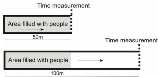
**Fig. 1.** Test 1. Geometry set up. Two corridors  $50 \times 2$  m and  $100 \times 2$  m in size, respectively, initial positions of people, and control lines.
