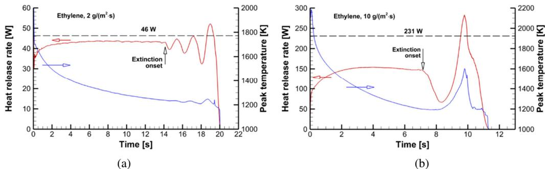
**Fig. 9.** Predicted transient variations of total heat release rate and peak temperature (100%  $C_2H_4$ , 21%  $O_2$ , 1 bar) at different fuel supply rates: (a)  $2\text{ g/(m}^2\cdot\text{s)}$ ; (b)  $10\text{ g/(m}^2\cdot\text{s)}$ . Dashed lines show the theoretical heat release rate in complete fuel oxidation.
