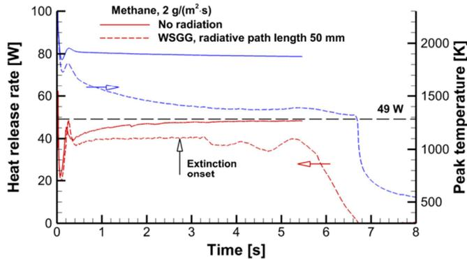
**Fig. 12.** Predicted transient variations of total heat release rate and peak temperature (100% CH<sub>4</sub>, 2 g/(m<sup>2</sup>·s), 21% O<sub>2</sub>, 1 bar) with and without radiative emission. Dashed line shows the theoretical heat release rate in complete fuel oxidation.
