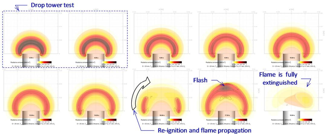
**Fig. 5.** Predicted temperature distributions and heat release rate iso-curves in the central plane at the time instants 2, 4, 6, 8, 10, 12, 14, 16, 17, and 18 s (100%  $C_2H_4$ ,  $3.48 \text{ g}/(\text{m}^2 \cdot \text{s})$ , 33%  $O_2$ , 0.7 bar).
