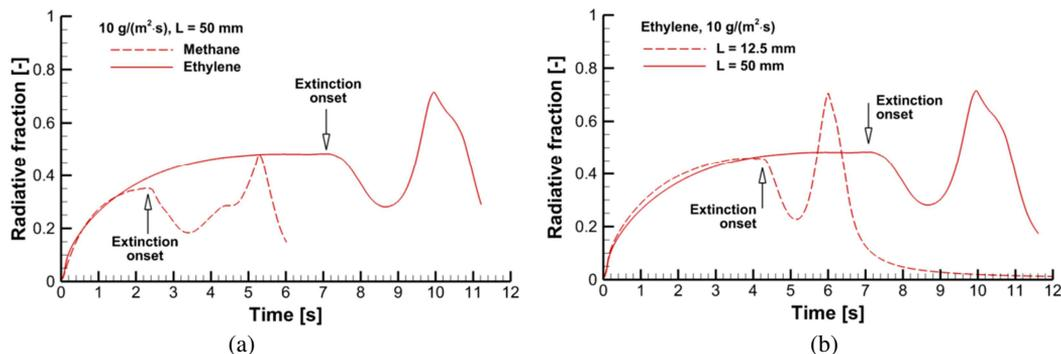
**Fig. 13.** Predicted transient variations of the radiative fraction (based on the theoretical heat release rate): (a) the effect of fuel; (b) the effect of mean radiation pathlength.
