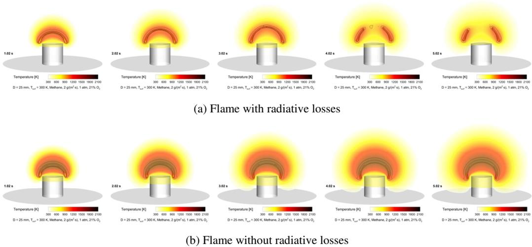
**Fig. 11.** Predicted temperature distributions and heat release rate iso-curves in the central plane at the time instants 1, 2, 3, 4, and 5 s (100% CH<sub>4</sub>, 2 g/(m<sup>2</sup>·s), 21% O<sub>2</sub>, 1 bar).
