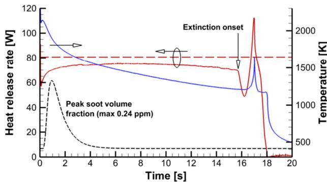
**Fig. 6.** Predicted transient variations of total heat release rate, peak temperature, and peak soot volume fraction (100%  $C_2H_4$ ,  $3.48 \text{ g}/(\text{m}^2 \cdot \text{s})$ , 33%  $O_2$ , 0.7 bar).
