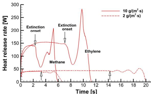
**Fig. 10.** Predicted transient variations of total heat release rate in methane and ethylene BRE flames at the fuel supply rates 2 and  $10\text{ g/(m}^2\cdot\text{s)}$ , 21%  $O_2$ , 1 bar. The arrows show the extinction onset.
