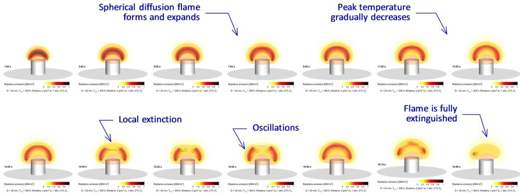
**Fig. 7.** Predicted temperature distributions and heat release rate iso-curves in the central plane at the time instants 1, 3, 5, 7, 9, 11, 13, 14, 14.5, 15, 19, 19.5, 19.7, and 19.9 s (100% C<sub>2</sub>H<sub>4</sub>, 2 g/(m<sup>2</sup>·s), 21% O<sub>2</sub>, 1 bar).
