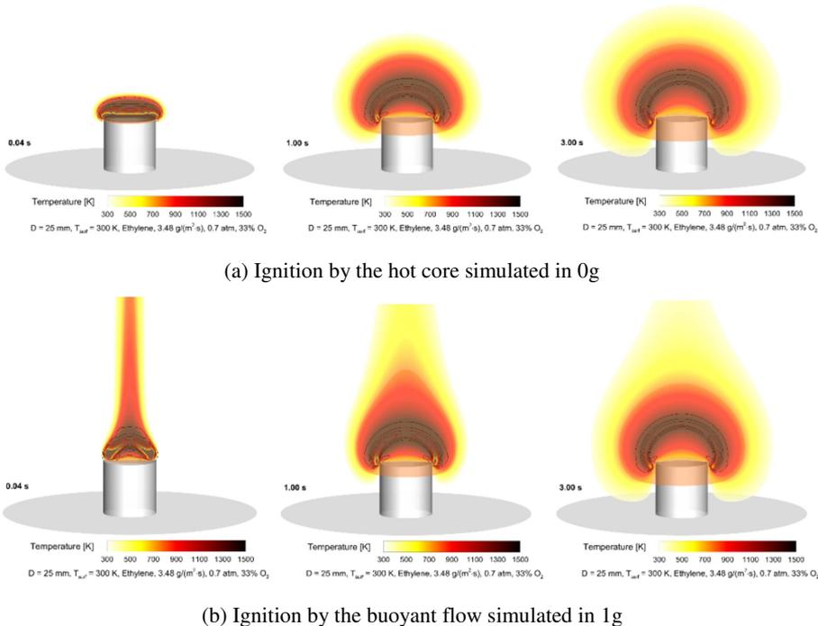
**Fig. 2.** Instantaneous flame structure at time instants 0.04, 1 and 3 s (left to right) shown by the temperature distribution and the iso-curves of the heat release rate (solid lines) in the axial plane. Simulation results are presented for two methods of ignition.
