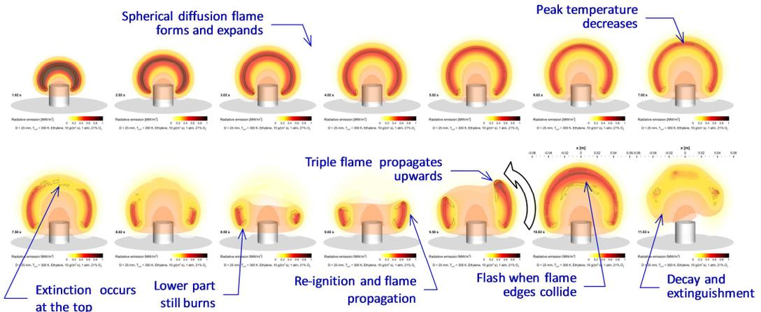
**Fig. 8.** Predicted temperature distributions and heat release rate iso-curves in the central plane at the time instants 1, 2, 3, 4, 5, 6, 7, 7.5, 8, 8.5, 9, 9.5, 10, and 11 s (100% C<sub>2</sub>H<sub>4</sub>, 10 g/(m<sup>2</sup>·s), 21% O<sub>2</sub>, 1 bar).
