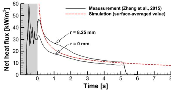
**Fig. 4.** Transient variation of the net heat flux at the burner surface. 100%  $\text{C}_2\text{H}_4$ ,  $3.48 \text{ g}/(\text{m}^2 \cdot \text{s})$ , 33%  $\text{O}_2$ , 0.7 bar.
