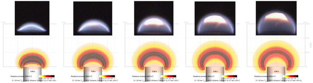
**Fig. 3.** Drop tower microgravity test with 100%  $\text{C}_2\text{H}_4$ ,  $3.48 \text{ g}/(\text{m}^2 \cdot \text{s})$ , 33%  $\text{O}_2$ , 0.7 bar. Upper photos: experimental images at time instants 0.5, 1.5, 2.5, 3.5, and 4.5 s [2]. Lower plots – predicted temperature distributions and heat release rate iso-curves in the central plane at the same time instants.
