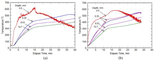
Fig. 4. Temporal variations of the temperature in the interior of the horizontally orientated specimen. (a) Flaming and (b) Non-flaming.
