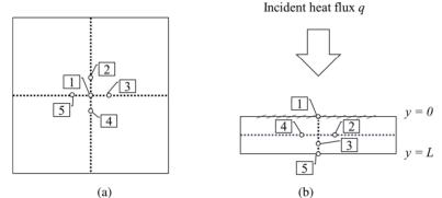
Fig. 1. Thermocouple set up in a specimen oriented horizontally (with a vertical radiant flux from the cone heater. (a) top view; (b) cross-section view.
