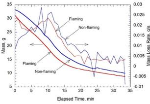
Fig. 6. Specimen mass and mass loss rate for flaming and non-flaming cases. The mass is presented at 1Hz, and mass loss rate is shown at 1/60Hz due to load cell sensitivity.
