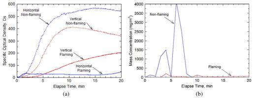
Fig. 2. Temporal variations of (a) the specific optical density (vertical and horizontal specimen) and (b) the particulate mass concentration (horizontal specimen).
