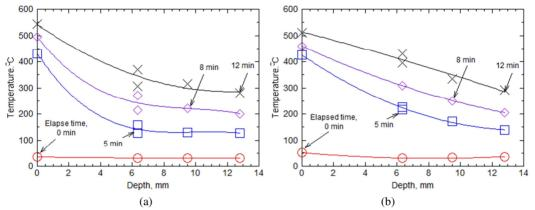
Fig. 5. Temperature in the interior of the horizontally orientated specimen. (a) Flaming and (b) Non-flaming.
