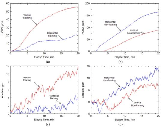
**Fig. 3.** Temporal variations of (a, b) formaldehyde and (c, d) acrolein concentrations. (a, c) Flaming and (b, d) non-flaming cases. Negative values indicate concentrations are too low for FTIR to read accurately.
