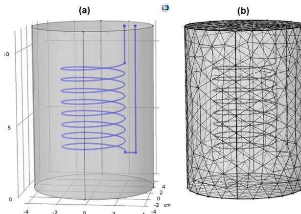
**Fig. 2.** The geometrical layout for the reactor vessel (a) and mesh used in the simulation (b)
