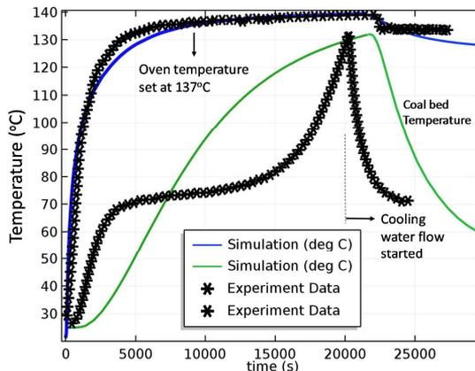
Fig. 10. Comparison between the simulation and experimental results at oven temperature 137 °C.
