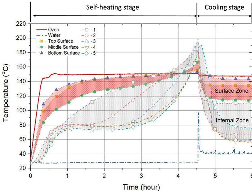
**Fig. 5.** Temperatures time history of a typical run at 147 °C oven temperature, using a 85 mm diameter wire-mesh cylindrical reactor. Cooling begins when central temperature reaches 50°C above the oven temperature.
