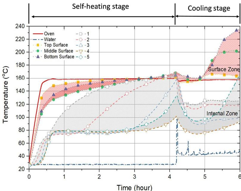
**Fig. 6.** Temperatures time history of a typical run at 157 °C oven temperature, a super-critical condition for spontaneous combustion.
