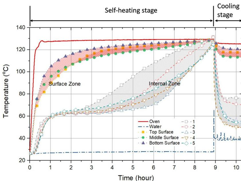
**Fig. 3** Temperatures time history of a typical run at 127 °C oven temperature, using a 100 mm diameter wire-mesh cylindrical reactor.
