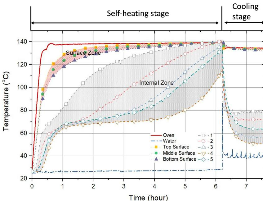
**Fig. 4.** Temperatures time history of a typical run at  $137^\circ\text{C}$  oven temperature, using a 85 mm diameter wire-mesh cylindrical reactor.
