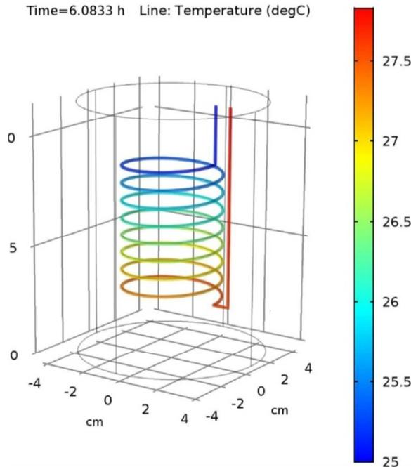
Fig. 9. Increase of cooling water temperatures during simulation in step 2.
