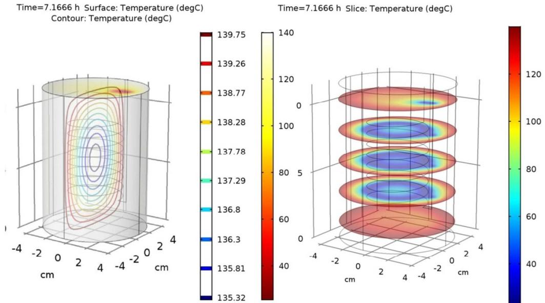
**Fig. 8.** Surface and contour temperatures during simulation in step 2.
