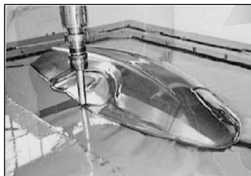
Fig. 2.19. Dieless NC forming process
