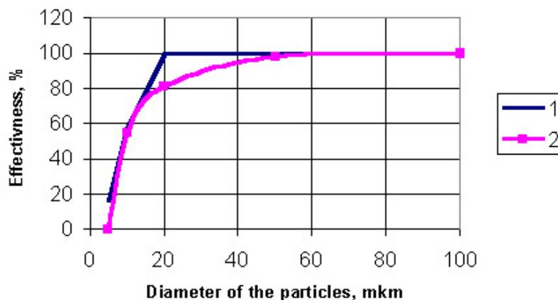
Fig. 3.1. Comparison of the effectiveness of separation received theoretically – 1, and experimentally – 2
