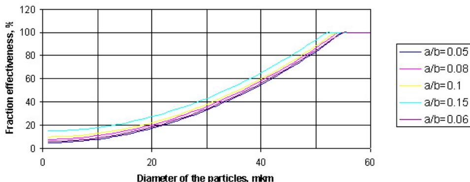
Fig. 2.6. Fraction effectiveness of the dust-collections in the curvilinear channel depending on the size of the dust extraction slits. (The calculations were made for the channel of unit width)
