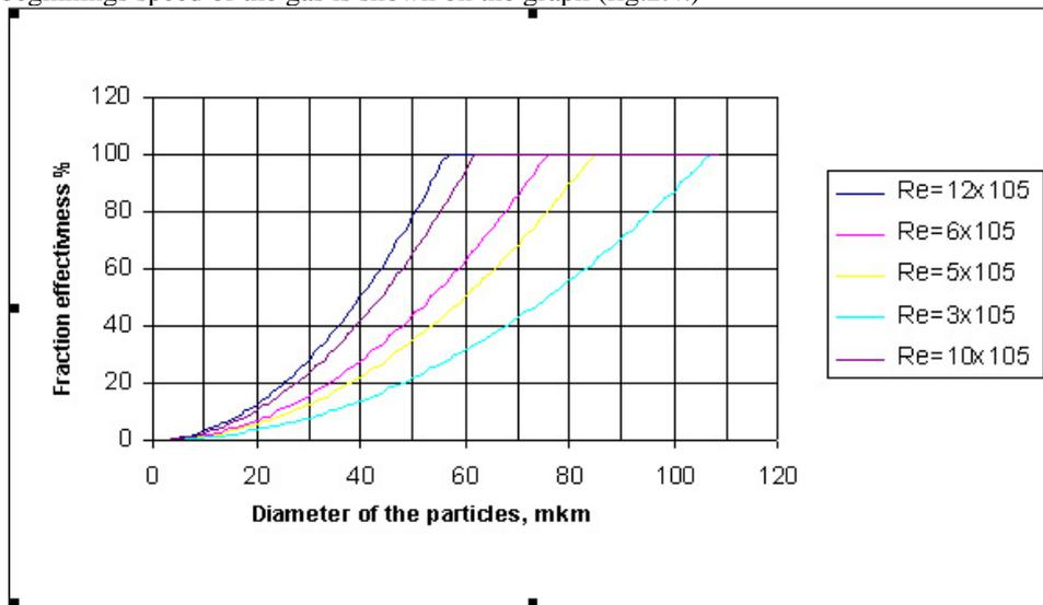
Fig. 2.4. Fraction effectiveness of the dust-collections in the curvilinear channel depending on the Reynolds number for the gas stream. (The calculations were made for the channel of unit width; density of the particles  $\rho = 2000 \text{ kg} / \text{m}^3$ ; - kinematics viscosity of the gas environment  $\mu = 22,2 \cdot 10^{-6} \text{ Nw} \cdot \text{sec}^2 / \text{m}^2$ .)
