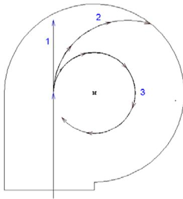
Fig. 0.1. Trajectories of the movement of dust particles
