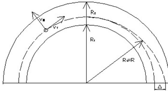
Fig.2.3. Movement on the single particle in the gas stream flowing in the concentric channel
