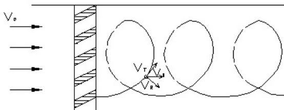
Fig.2.7. The scheme of the movement of the single particle in the direct-flow cyclone.
