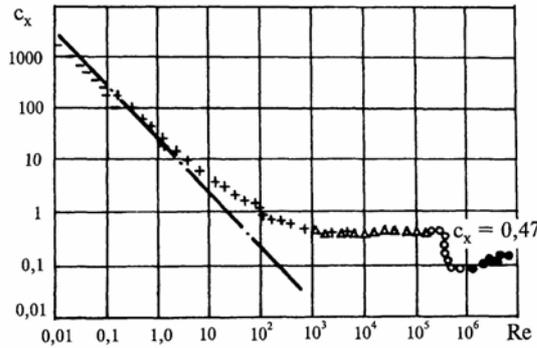
Fig. 2.2. Dependence of the coefficient of resistance of the sphere in the Reynolds number, and influence terms of the experiment into  $c_x$  near the critical Reynolds number.
