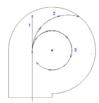
Fig. 0.1. Trajectories of the movement of dust particles
