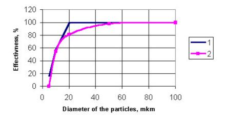
Fig. 3.1. Comparison of the effectiveness of separation received theoretically - 1, and experimentally -
