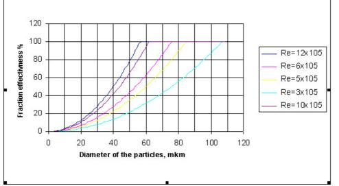
Fig. 2.4. Fraction effectiveness of the dust-collections in the curvilinear channel depending on the Reynolds number for the gas stream. (The calculations were made for the channel of unit width; density of the particles  $\rho = 2000 kg / m^3$ ; - kinematics viscosity of the gas environment  $\mu = 22, 2 \cdot 10^{-6} Nw \cdot \sec^2 / m^2$ .)
