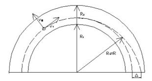
Fig.2.3. Movement on the single particle in the gas stream flowing in the concentric channel
